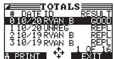
To select an item, the **UP (▲)** or **DOWN (▼) ARROW** key to highlight the item, and press the appropriate soft key.
