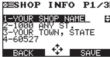
Use the **UP (▲)** or **DOWN (▼) ARROW** keys to highlight a line for editing. Display the character, symbol, or number you want by rapidly pressing its key as many times as needed. If you pause, the cursor moves to the right. To backspace, press the **LEFT (◀) ARROW** key. Use the **RIGHT ARROW** key to add a space. Use the **UP/DOWN ARROW** keys to highlight a line for editing. When finished, press the appropriate soft key to save your settings.
