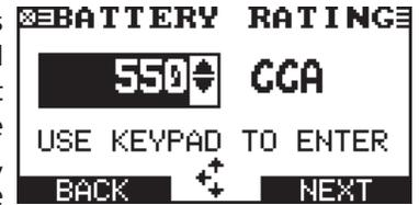
To select, use the **UP (▲)** or **DOWN (▼) ARROW** key to scroll to the value, or use the keypad to enter the value directly, and press the appropriate soft key. In the illustration the left directional arrow indicates that you can press the **LEFT (◀) ARROW** key to clear all or part of the entry.
